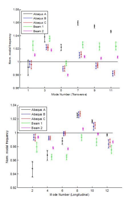
Figure 3: Uncertainty propagation to the output modal frequencies. Abaqus  $A \equiv FE - 1$ ,  $B \equiv FE - 2$ ,  $C \equiv FE - 3$ , Beam  $1 \equiv Beam - Fixed$ , Beam  $2 \equiv Beam - Flex$
